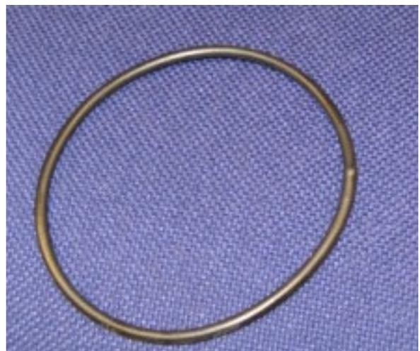
FIGURE 8 – LOOSE O-RING BLISTER AT 3 O'CLOCK POSITION
