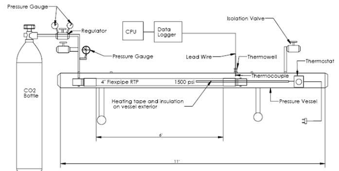
FIGURE 5 – EXPERIMENTAL TEST SET-UP
