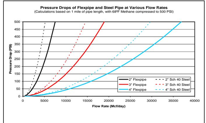
FIGURE 1 - REPRESENTATIVE PRESSURE DROPS FOR FLEXPIPE RTP VERSUS STEEL PIPE
