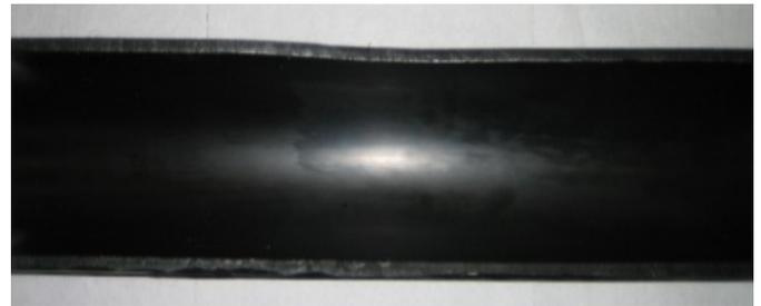
FIGURE 7 – INNER LINER SURFACE AFTER MULTIPLE CYCLES
