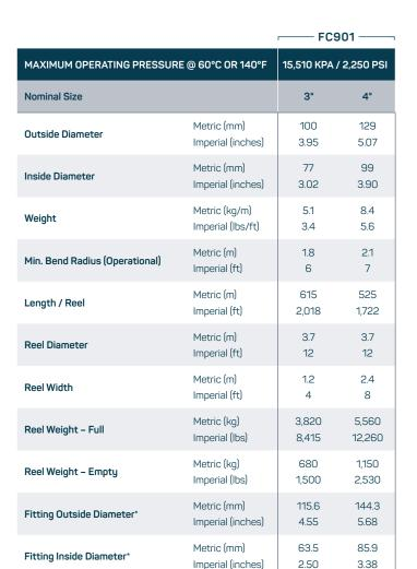
Lengths and weights are approximate as they may vary depending on the manufacturing run. \*Fitting dimensions do not include O.D. of flange provided for flanged end fittings. Fitting O.D. and I.D. apply to flanged end, weld-neck and pipe-to-pipe coupling fittings.
