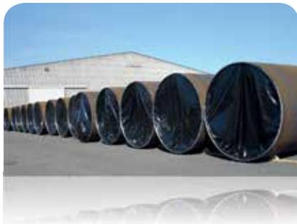
PVC Sheets on Ø 84" pipes
