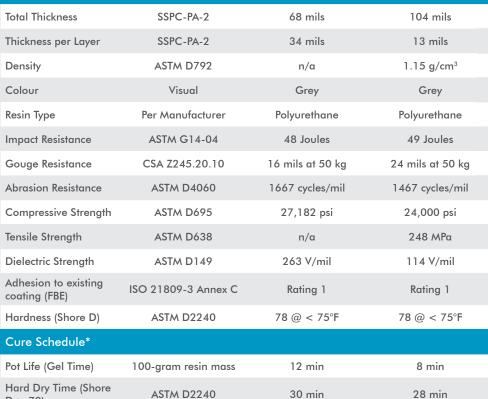
\*Cure times were tested at an ambient temperature of 24°C (75°F).
